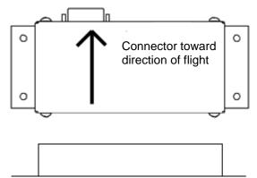
Connector forward and tabs mounted down
