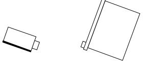
Side view of EDC-D10A, tabs mounted down and aligned within 1 degree of pitch with EFIS-D100
