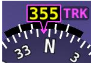
Figure 17 – GPS Track substitute for Magnetic Heading
