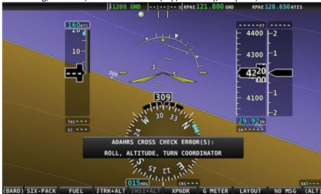
Figure 26 – ADAHRS Cross-Checking Disagreement
