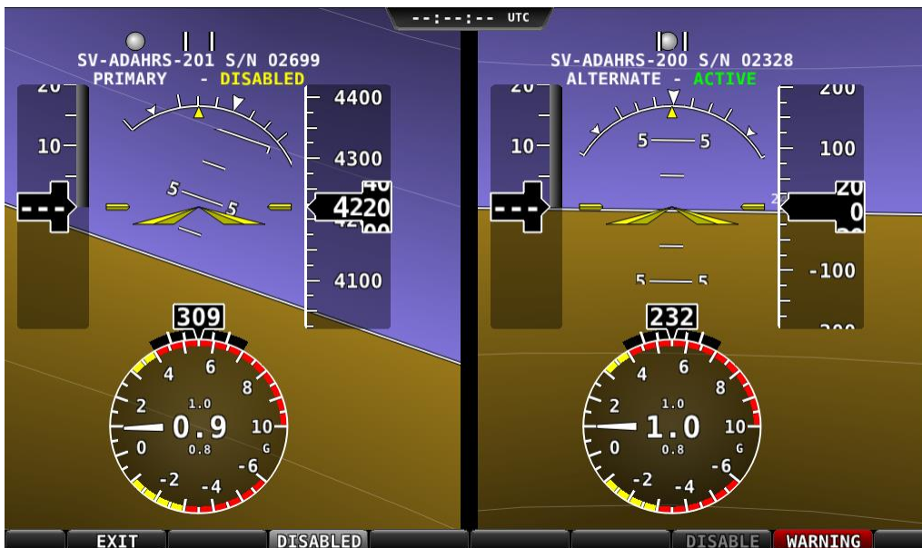
Figure 28 – ADAHRS Cross-Check Comparison (one ADAHRS disabled)
