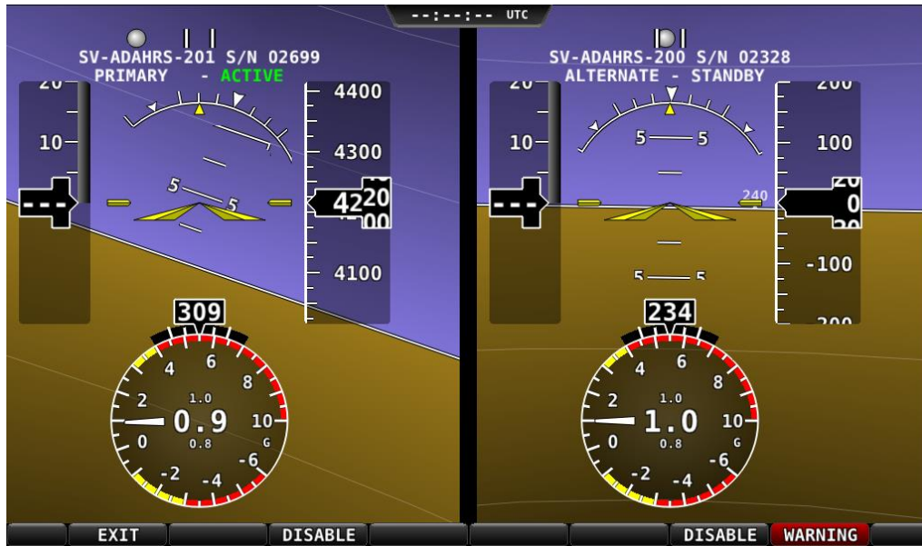
Figure 27 – ADAHRS Cross-Check Comparison
