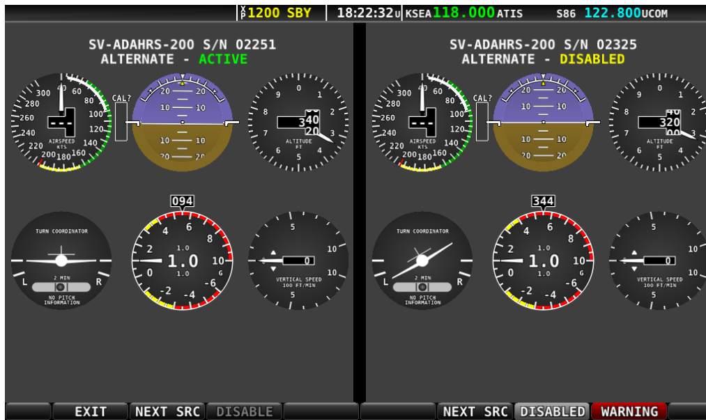
Figure 29 –ADAHRS Cross-Check Comparison – SIX-PACK
