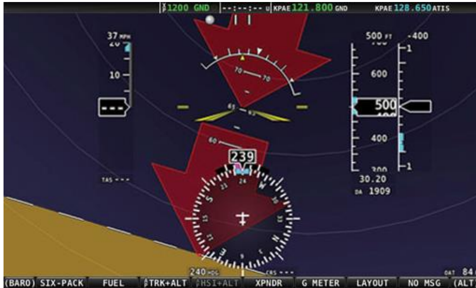
Figure 24 – Extreme Pitch Warning Indicator Arrows
