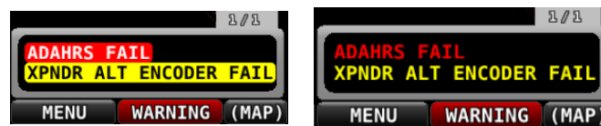
Figure 109 – Unacknowledged (left) and Acknowledged (right) Alarms
