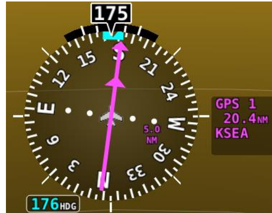
Figure 18 – HSI Displaying GPS
