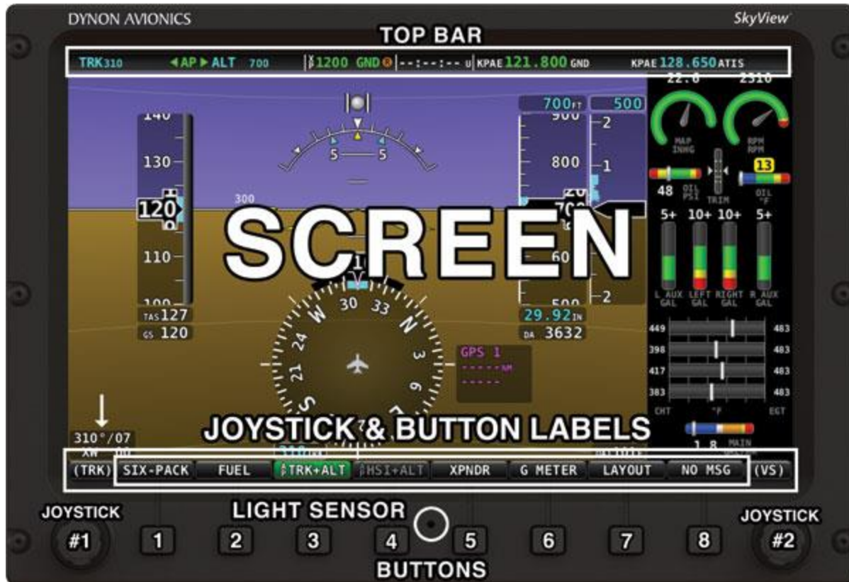
Figure 1 – SkyView SE Display Front Bezel Layout
