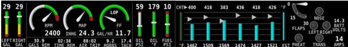
Figure 22: Example of Engine Bottom Band Layout for Single-engine Monitoring
