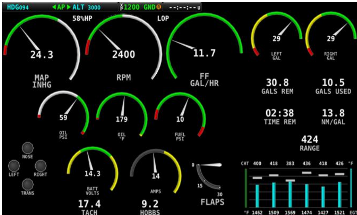
Figure 17: Example of 100% Page Layout for Single-engine Monitoring
