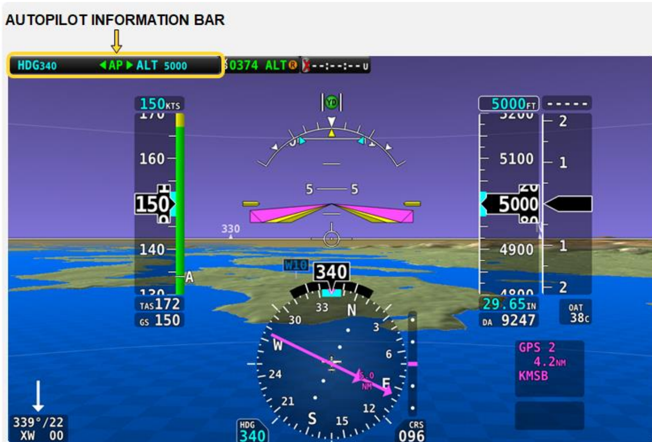
Figure 33: Autopilot Information Bar
