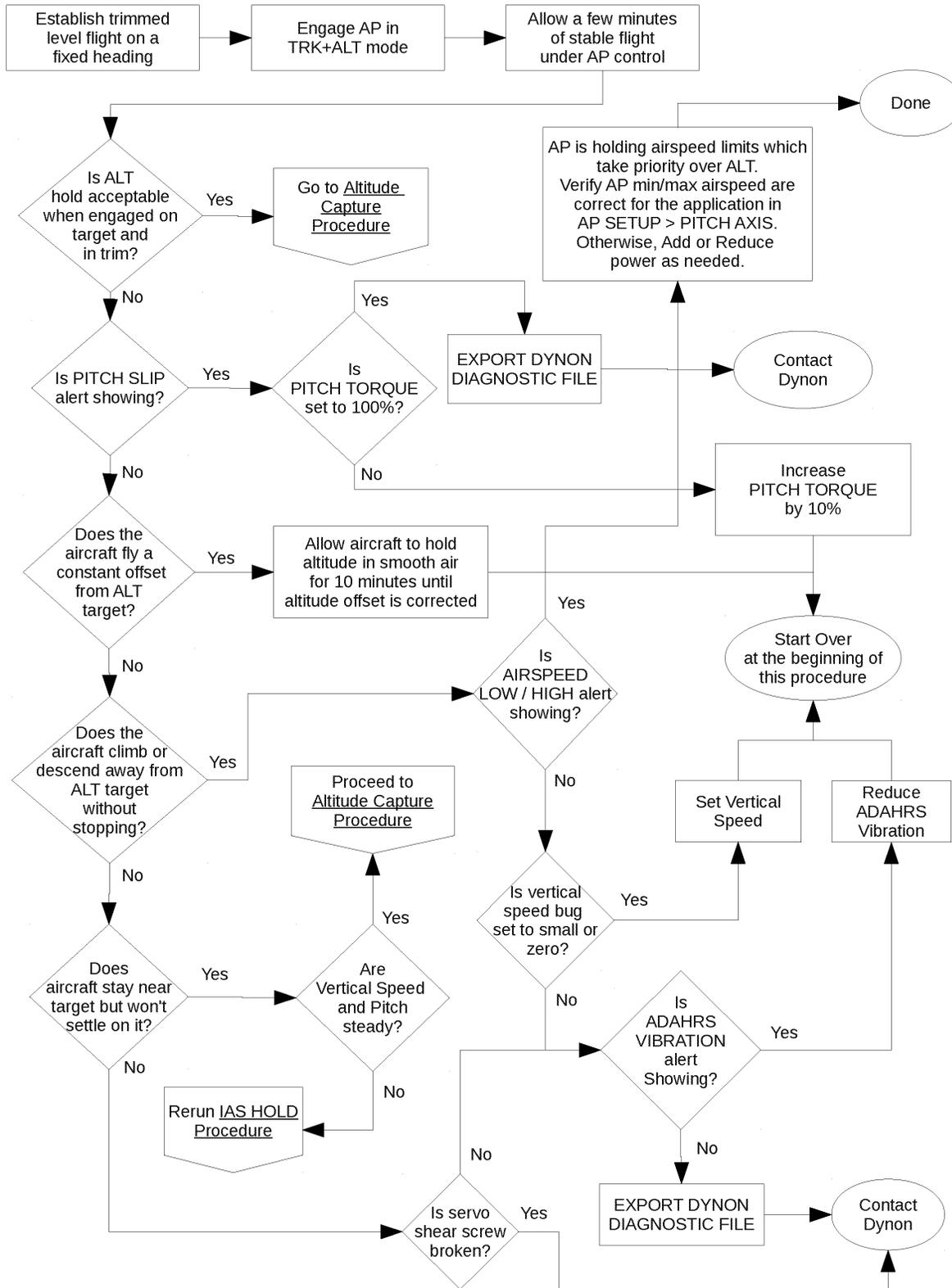
Figure 3 – Pitch Axis – Altitude Hold Procedure
