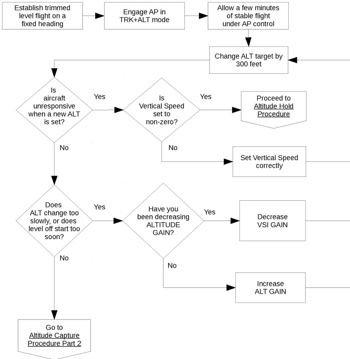
Figure 4 – Altitude Capture Procedure (Part 1 of 2)
