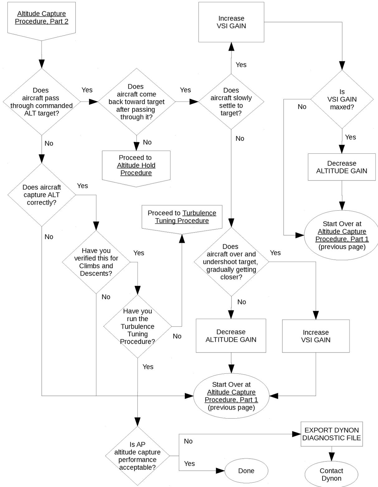
Figure 5 – Altitude Capture Procedure (Part 2 of 2)
