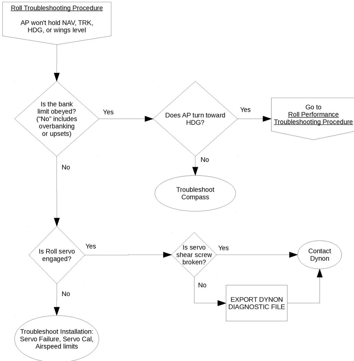
Figure 7 – Roll Axis – Roll Troubleshooting Procedure
