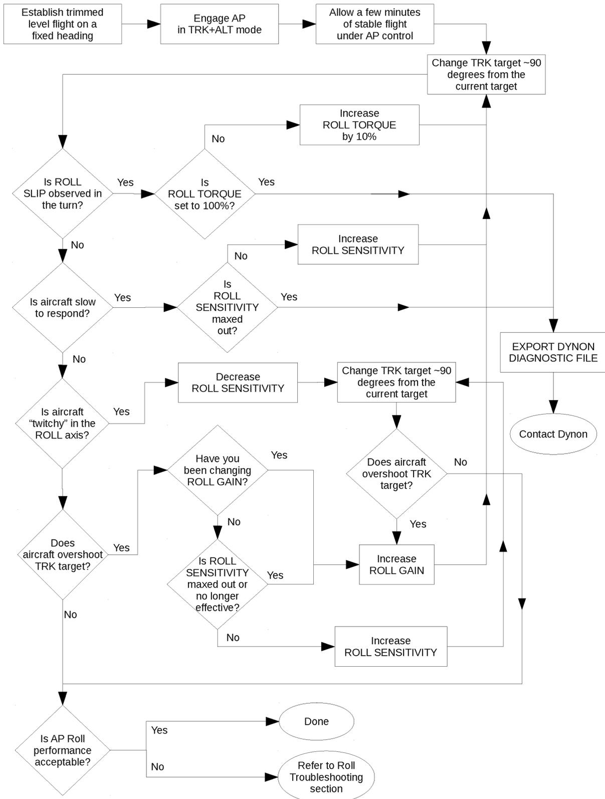
Figure 1 – Roll Axis – TRK and Turns Procedure
