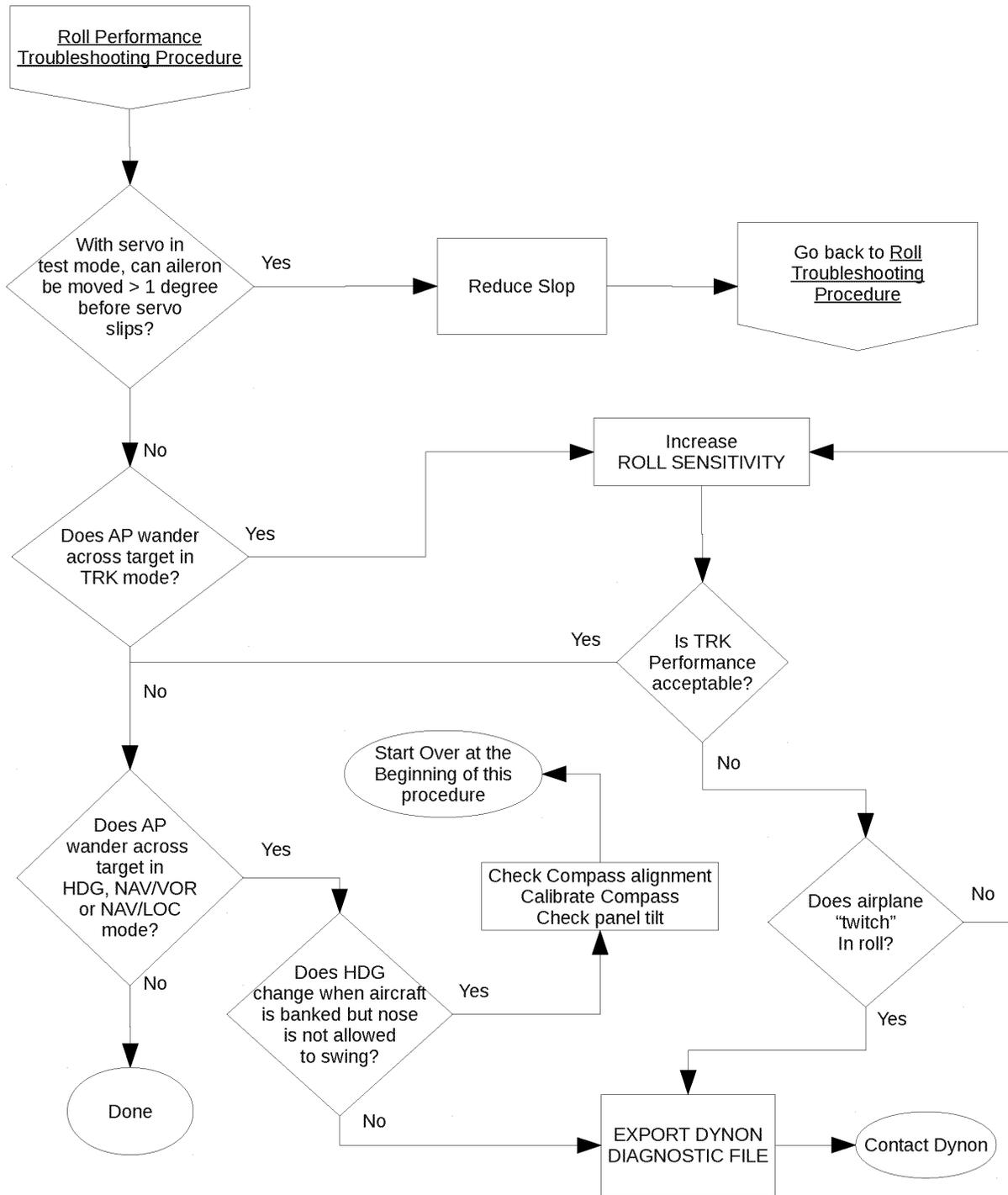
Figure 8 – Roll Axis – Roll Performance Troubleshooting Procedure
