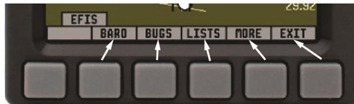
Figure 3: EFIS-D10A Menu System
