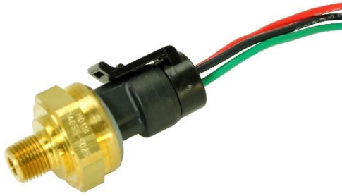
Figure 58 – Original 1/8-27 NPT 0-150 PSI Sensor (P/N 503388-000)
