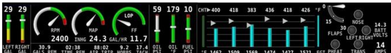
Figure 75 – Engine Bottom Band Layout for Single-engine Monitoring
