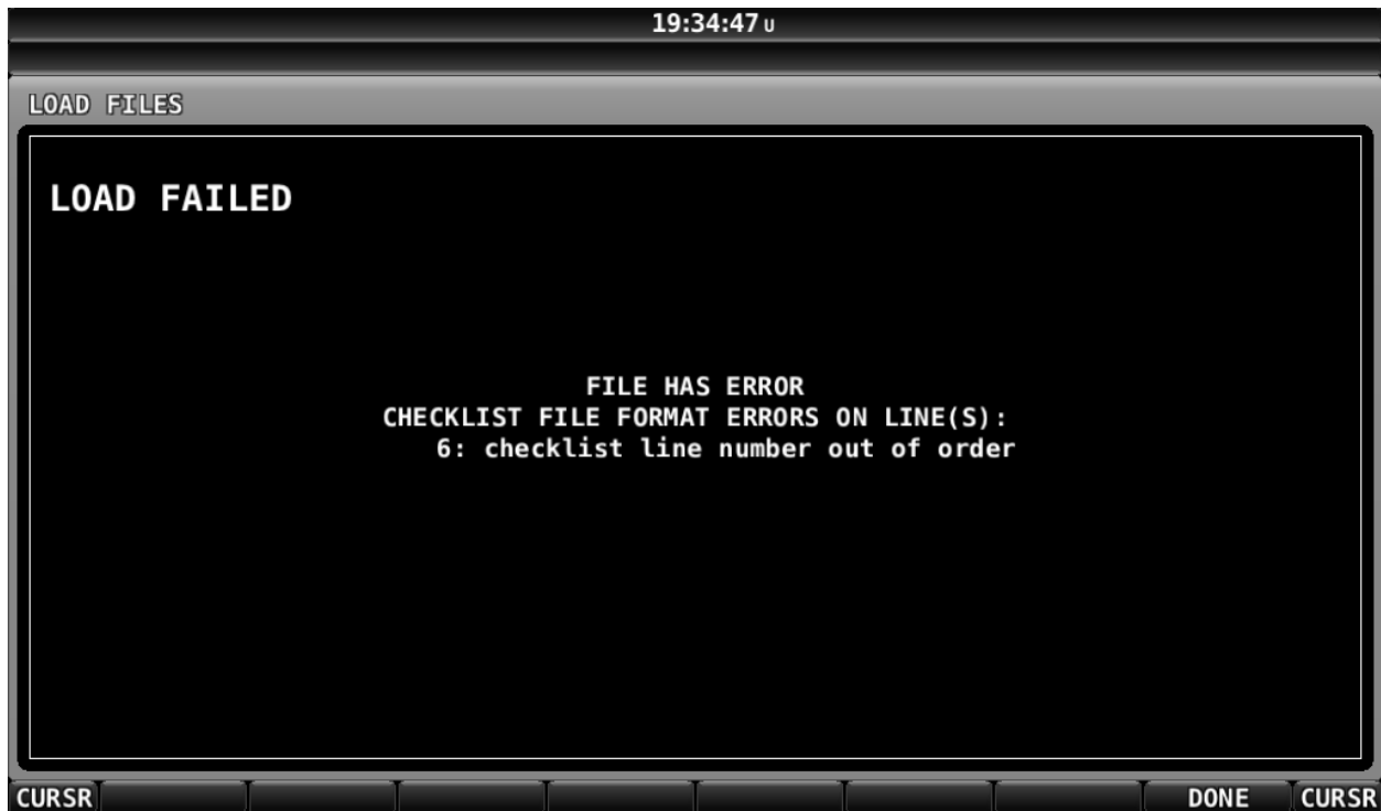
Figure 167: Checklist File Has an Error, Line Number Displayed, Could Not Be Loaded
