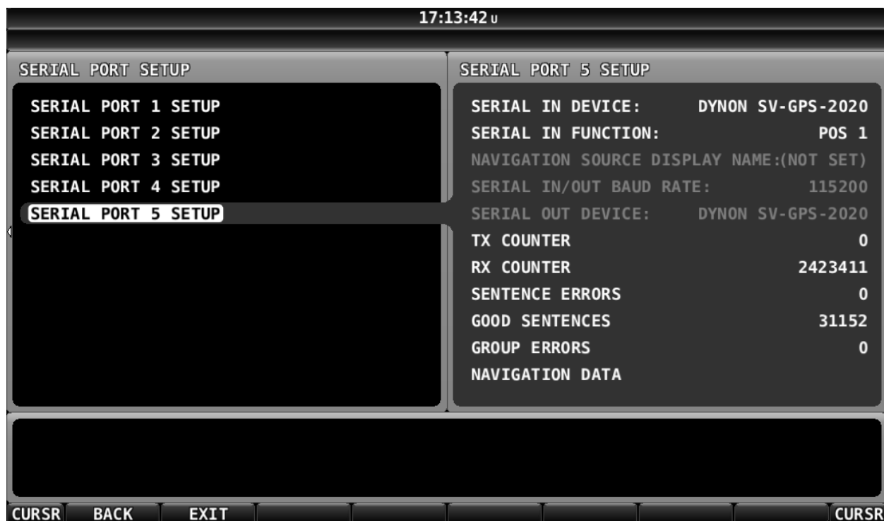
Figure 86: Serial Port 5 Setup for SV-GPS-2020
