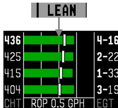
**In the above example, cylinder 3's EGT peaked first and cylinder 1's EGT peaked last. There was a total increase of 0.5 GPH in fuel flow between the first and last cylinder peak, indicating rich-of-peak operation.**
