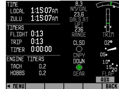
*When ENGINE TYPE is set to ROTAX (in EMS > SETUP > GLOBAL), only Hobbs time is displayed in the ENGINE TIMERS section; Tach time is not displayed, due to specific manufacturer recommendation.*
