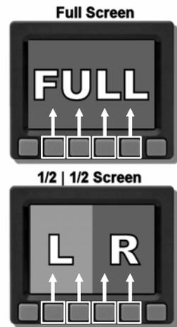
**The configuration of the pages on the screen determines which buttons are used to display a page's menu.**
