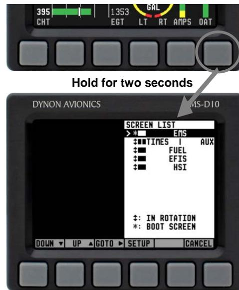
**With no menus displayed, pressing button six for two seconds displays the SCREEN LIST menu, from which you may switch to, and set up, various screen configurations.**
