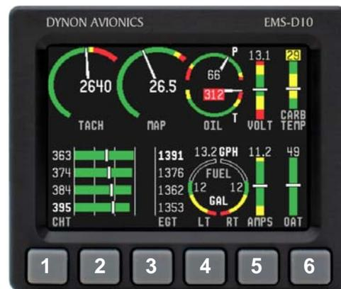
**User interaction takes place via the EMS-D120 main display and the six buttons beneath. Note: buttons are not labeled on actual product**
