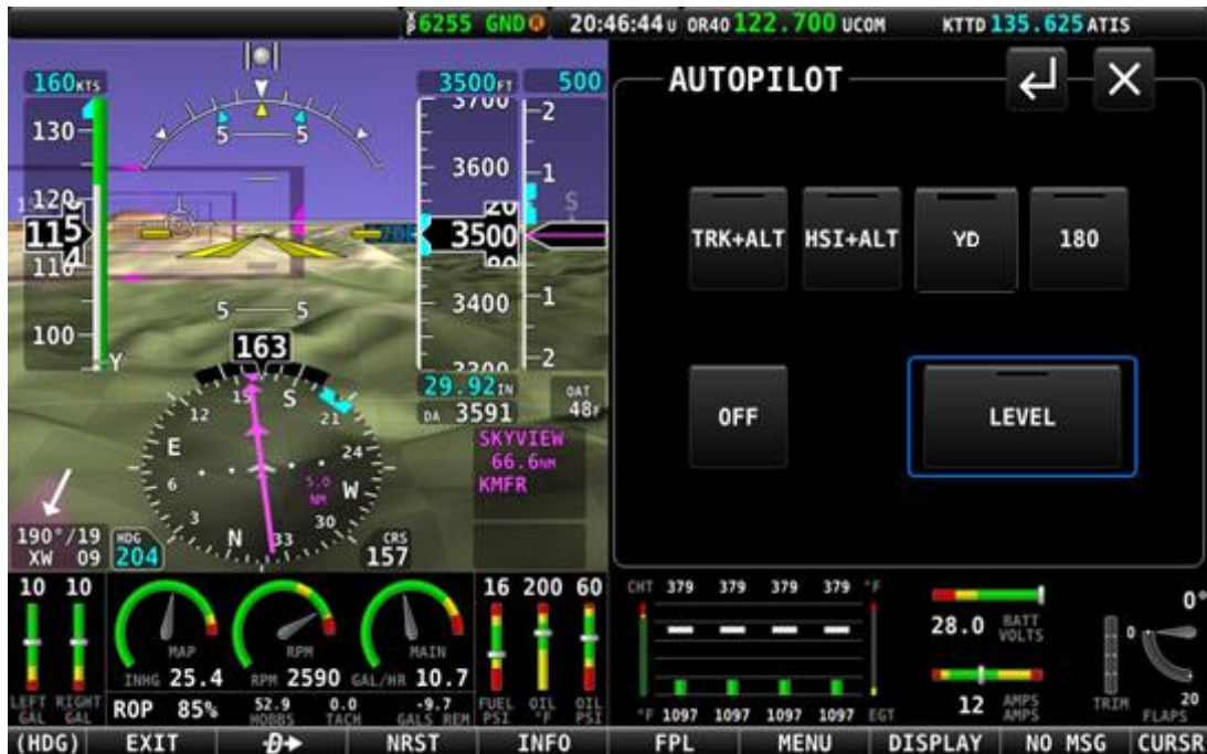
Figure 224 – AUTOPILOT Control page – Simplified Control Scheme
