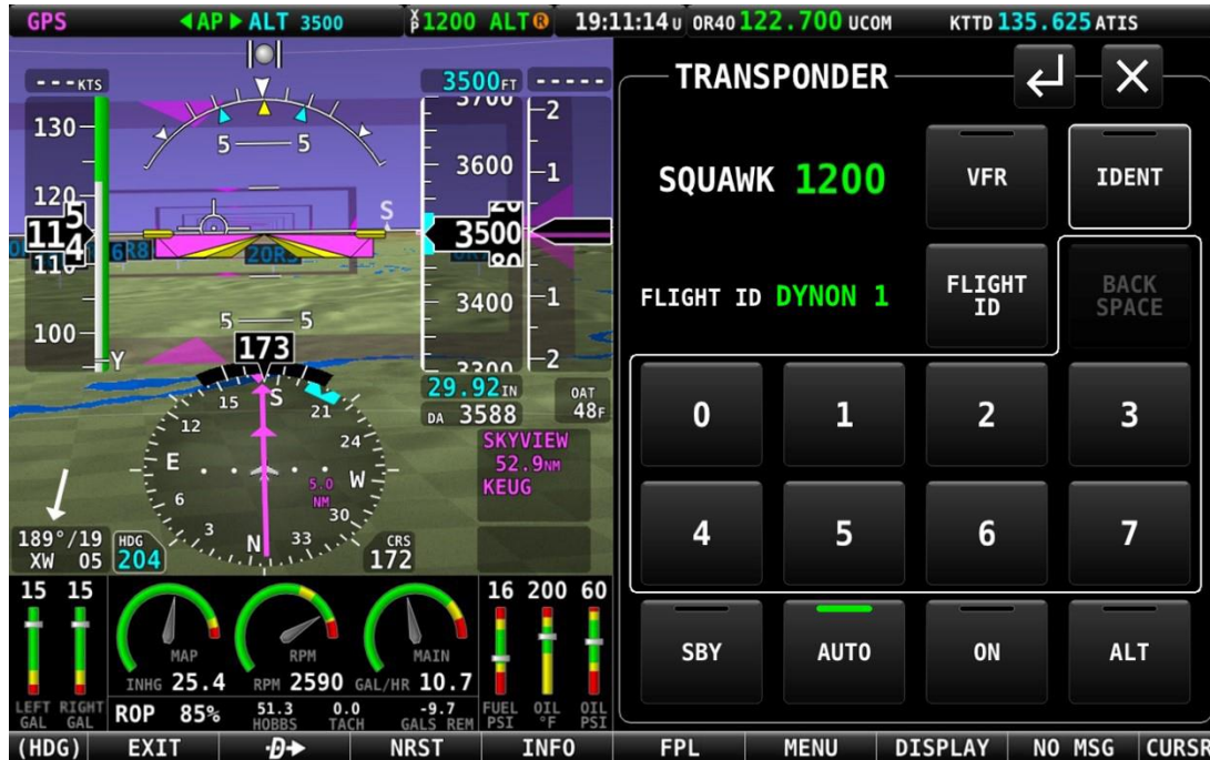
Figure 209 – TRANSPONDER control page
