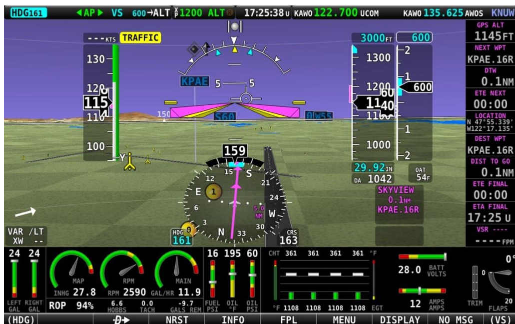
Figure 69 – SkyView HDX Synthetic Vision Traffic Alert
