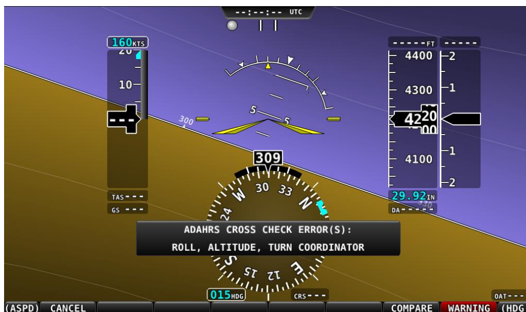
Figure 87 – ADAHRS Cross-Checking Disagreement
