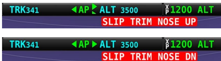
Figure 213 – Pitch Slip Trim Nose Up and Down Alerts
