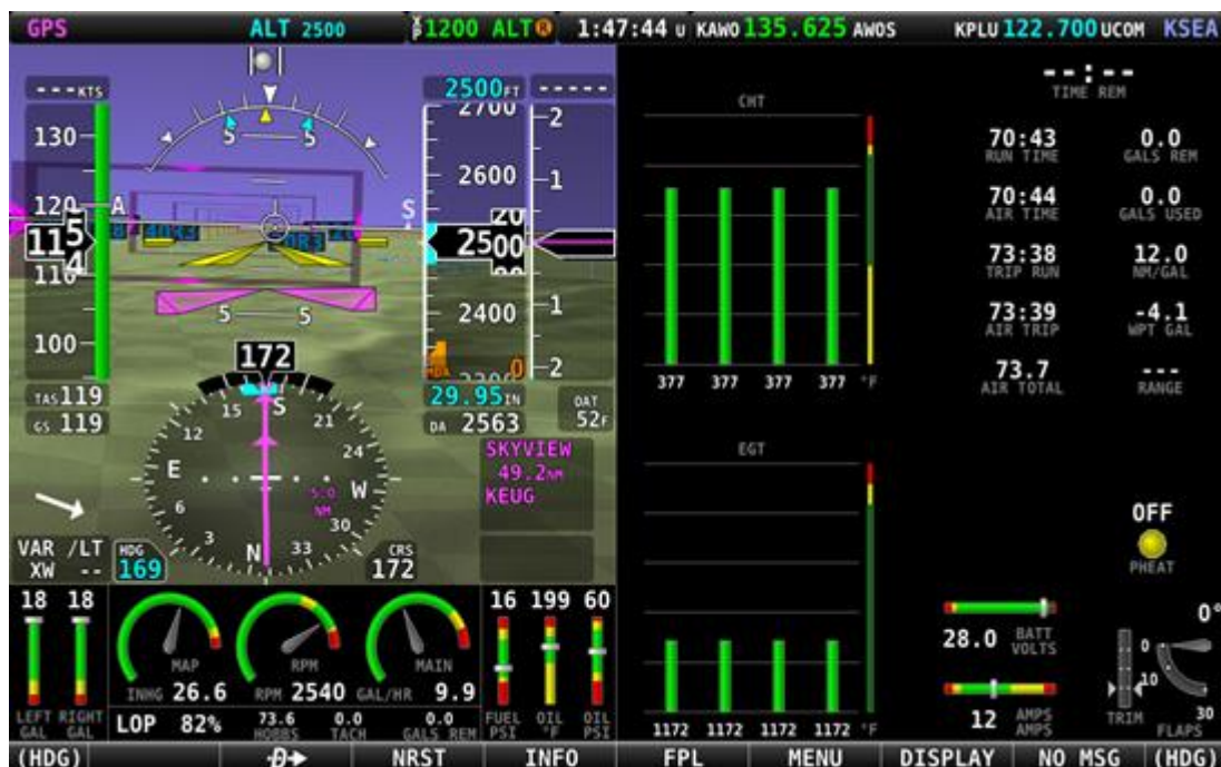
Figure 15 – 50% PFD / 50% ENGINE with ENGINE BOTTOM BAND
