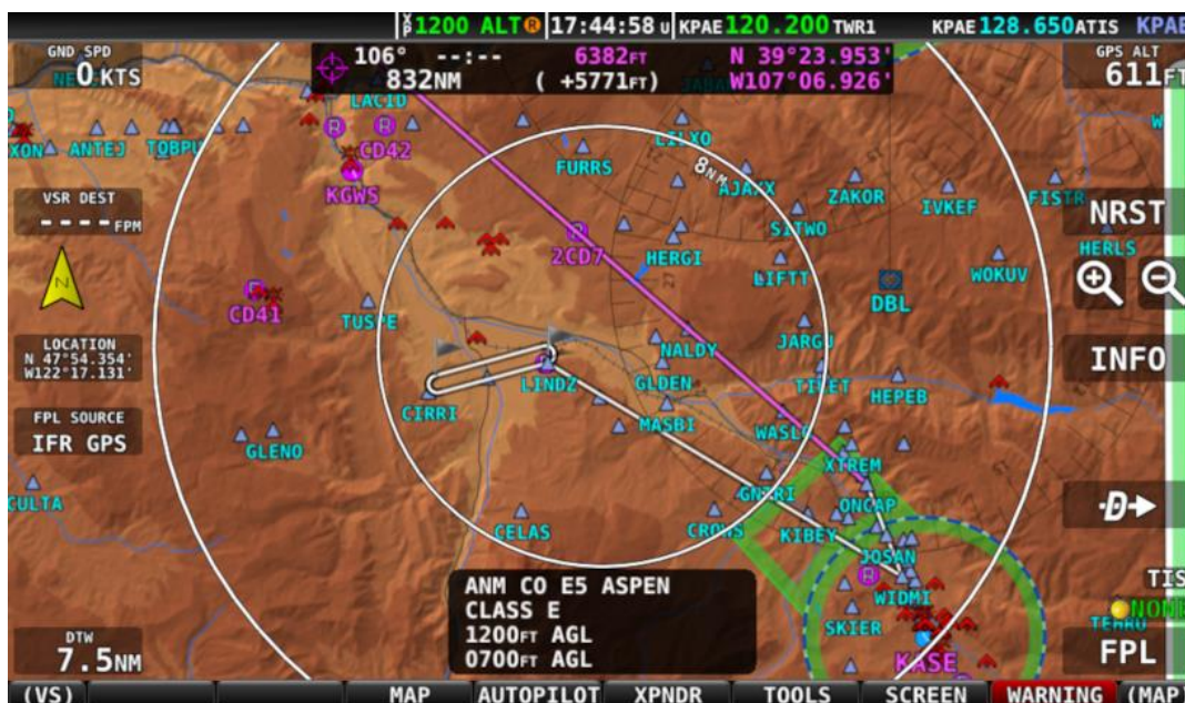
Figure 156 – Example of External Flight Plan Echo
