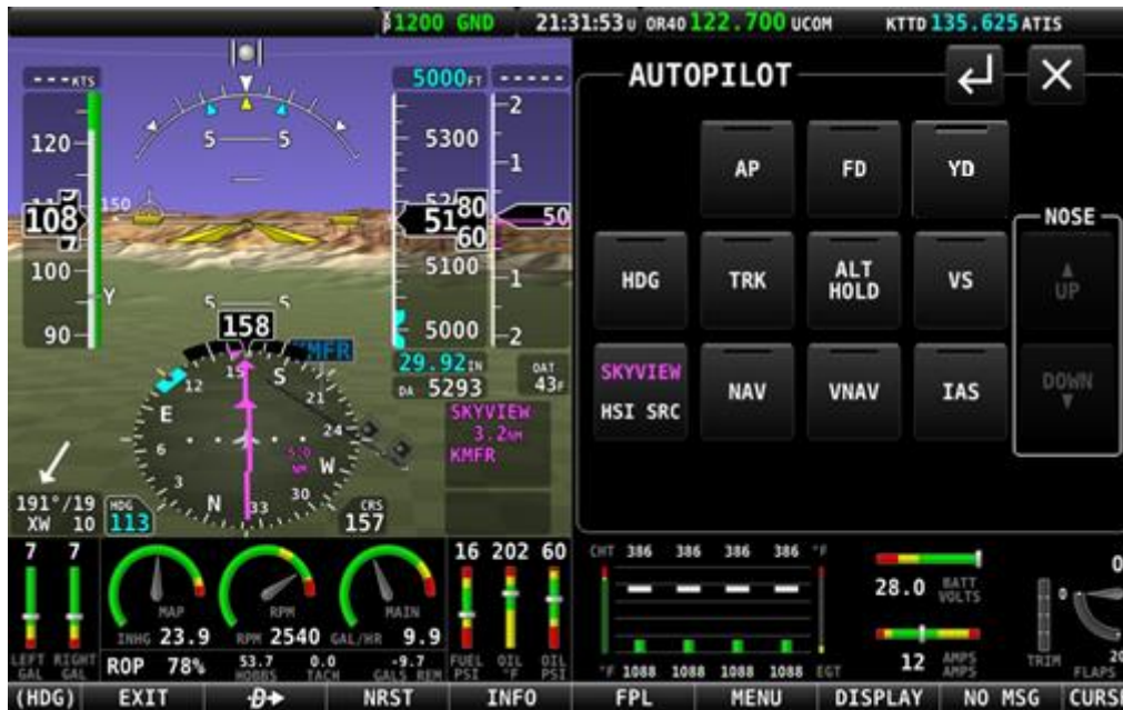
Figure 231 – AUTOPILOT Control page – Expert Control Scheme
