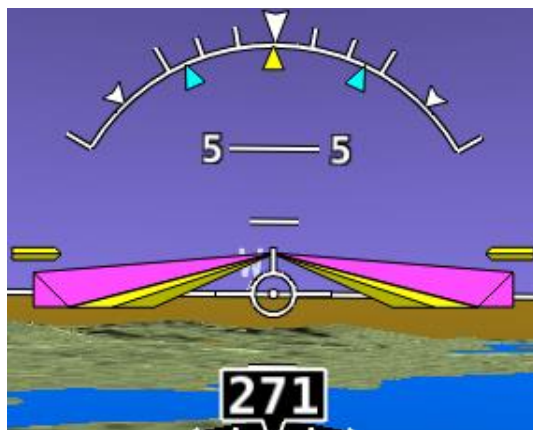
Figure 233 – Single Cue / Inverted-V with Autopilot Servos Engaged
