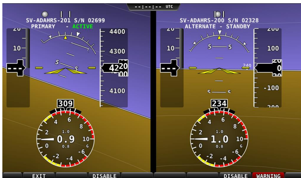
Figure 88 – ADAHRS Cross-Check Comparison (EFIS Presentation)
