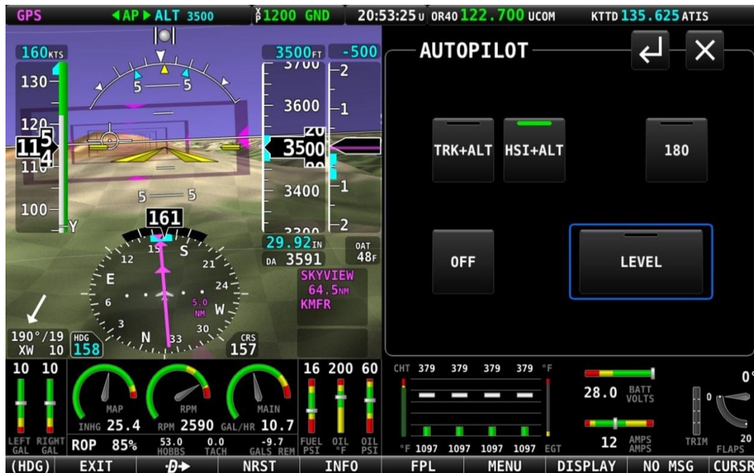
Figure 226 – HSI+ALT mode is engaged
