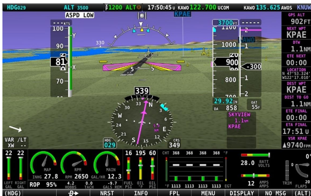
Figure 68 – SkyView HDX Synthetic Vision With Runways
