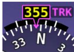
Figure 41 – GPS Track substitute for Magnetic Heading
