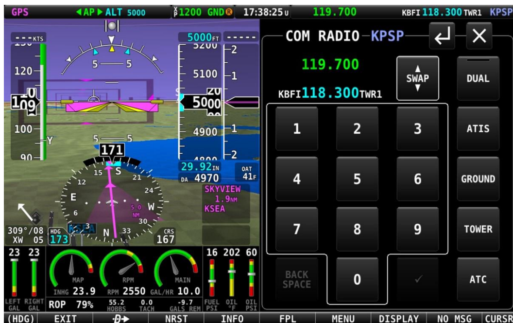
Figure 242 – Com Radio Control Panel
