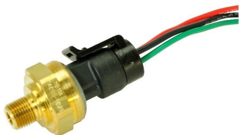
Figure 78 – Original 1/8-27 NPT 0-150 PSI Sensor (P/N 101693-000)
