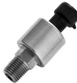
Figure 85 – New 1/8-27 NPT 0.6-15 PSI Sensor (P/N°103755-000) (Shown Without Wiring Connector)
