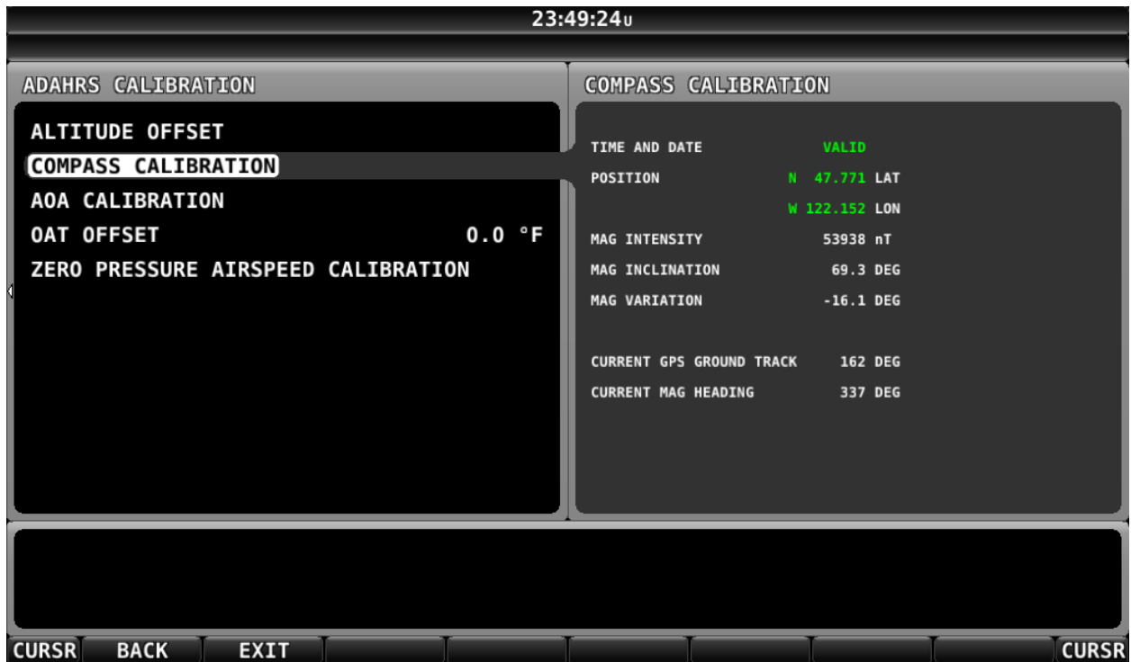
Figure 229 – On-ground COMPASS CALIBRATION Menu
