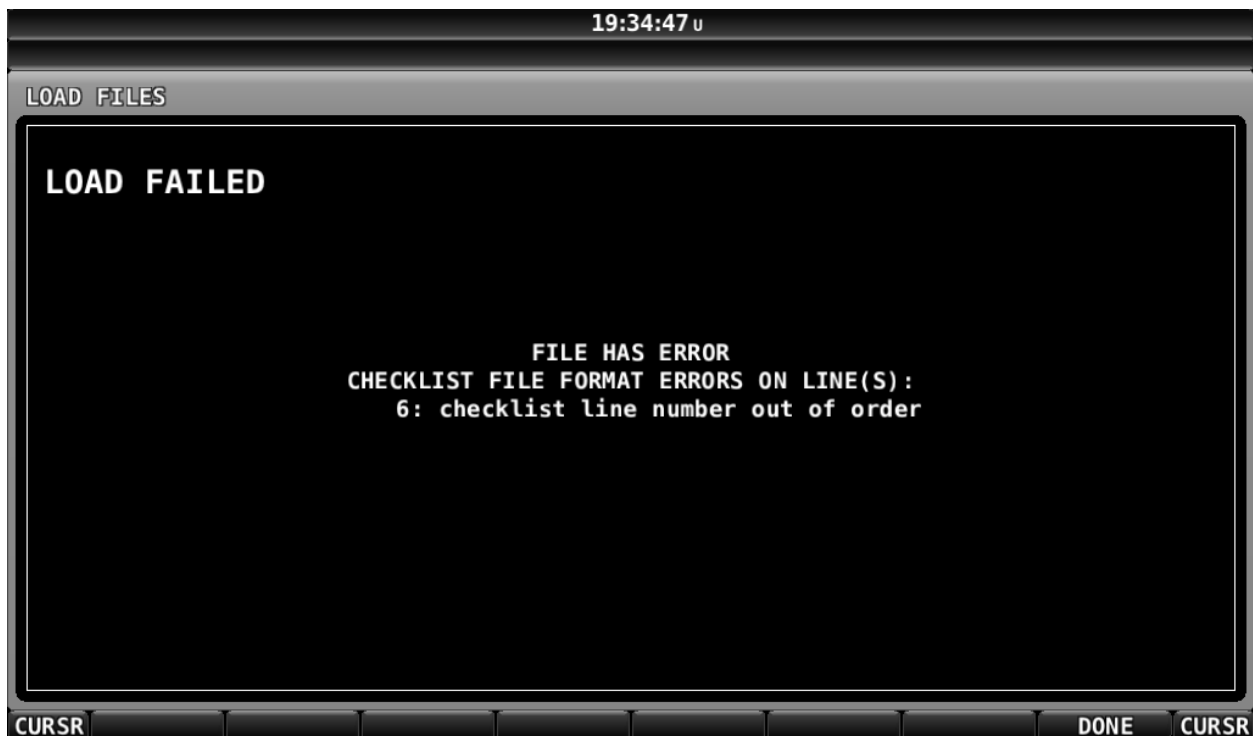
Figure 262 – Checklist File Has an Error, Line Number Displayed, Could Not Be Loaded
