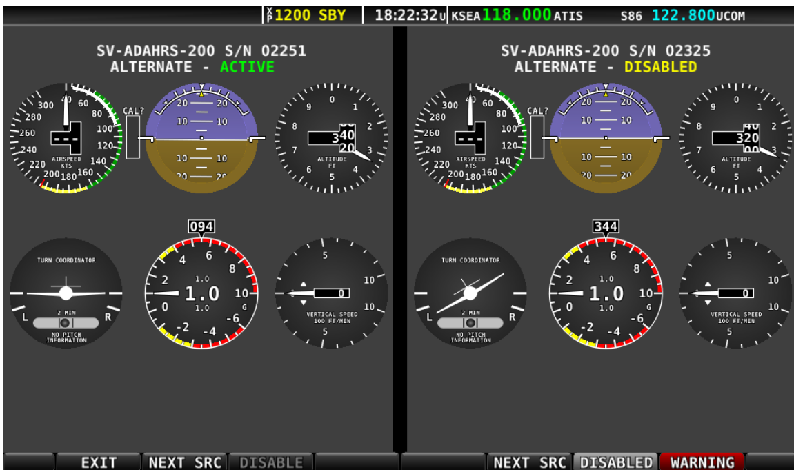
Figure 90: ADAHRS cross-check comparison (Six Pack presentation).
