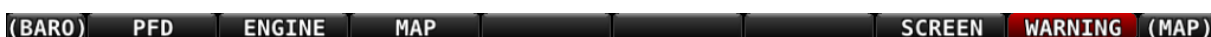
Figure 249: Message Notification Area above Button 8 (2nd from right), showing a Warning notification.
