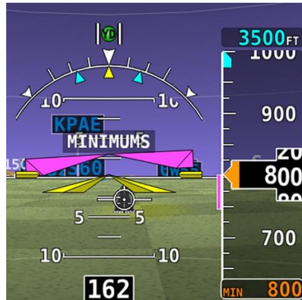
Figure 38: MIN Bug and "MINIMUMS" alert
