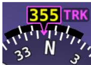
Figure 41: GPS Track substitute for Magnetic Heading indicator
