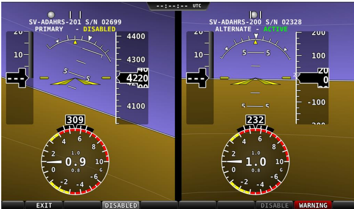
Figure 89: ADAHRS cross-check comparison (one ADAHRS disabled).
