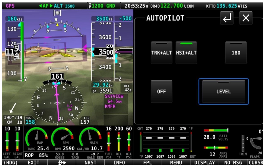
Figure 224: HSI+ALT Mode is engaged.
