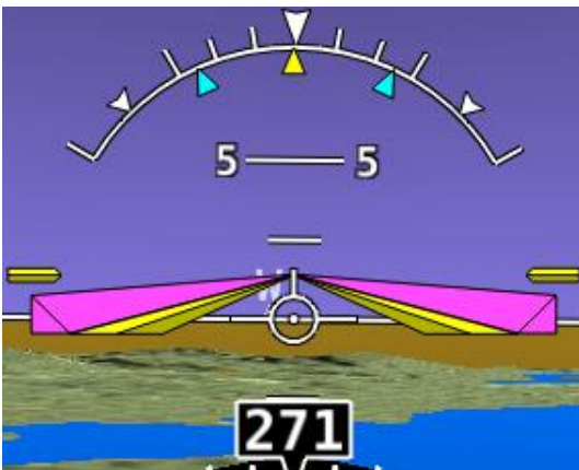
Figure 231: Single Cue / Inverted-V with Autopilot servos engaged.
