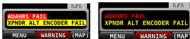
Figure 251: Unacknowledged (left) and Acknowledged (right) alerts
