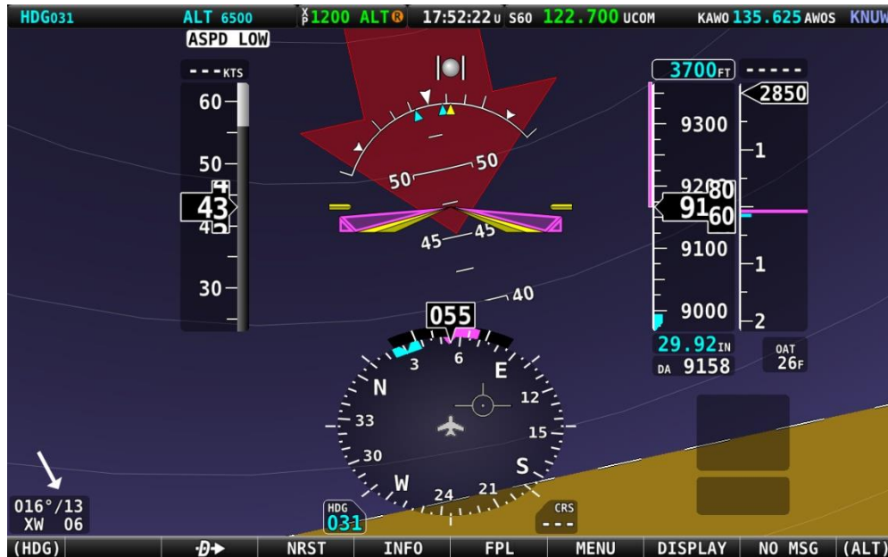
Figure 74: Extreme Pitch warning indicator arrows
