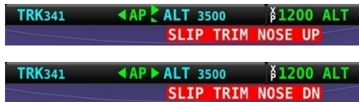
Figure 210: Pitch Slip Trim Nose Up and Down alerts
