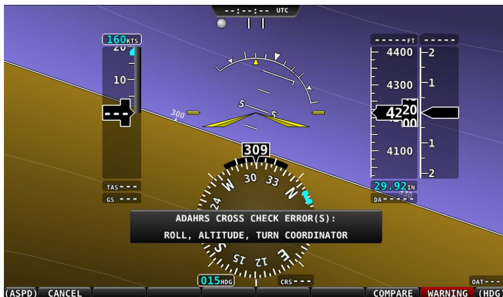
Figure 87: ADAHRS cross-checking disagreement.
